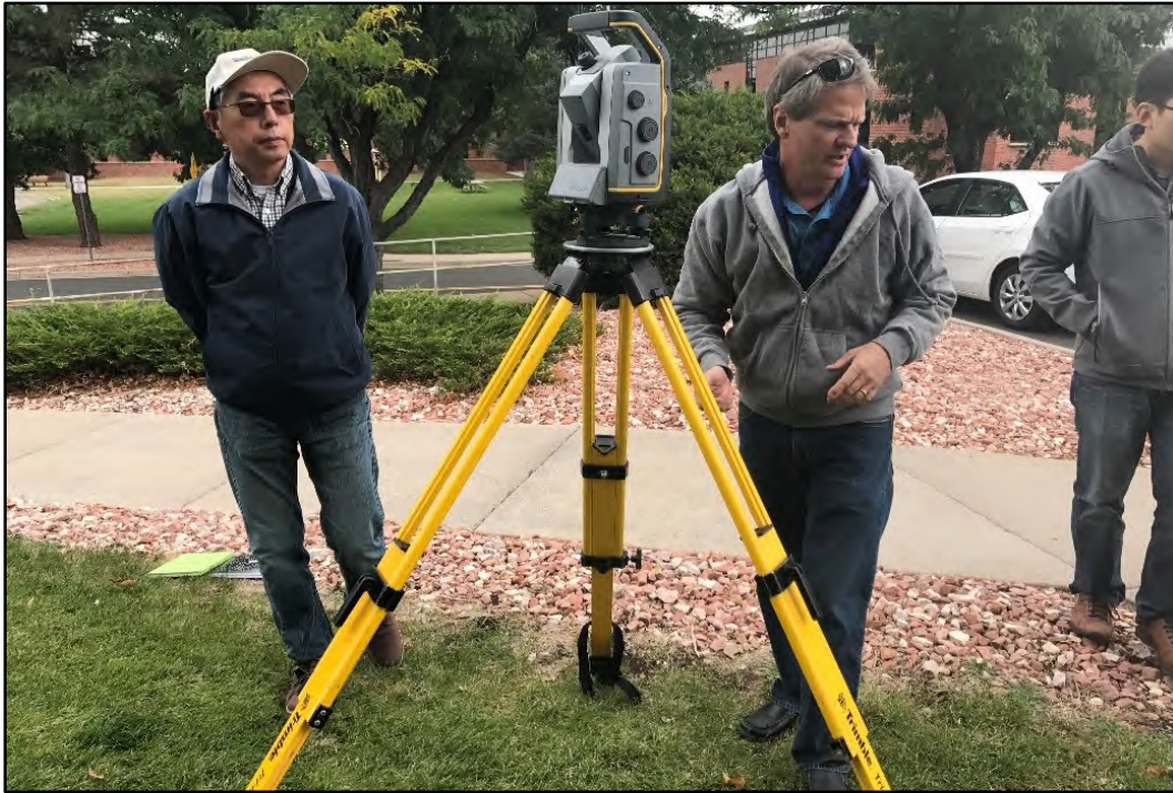
Figure 1.—Total station final setup.
