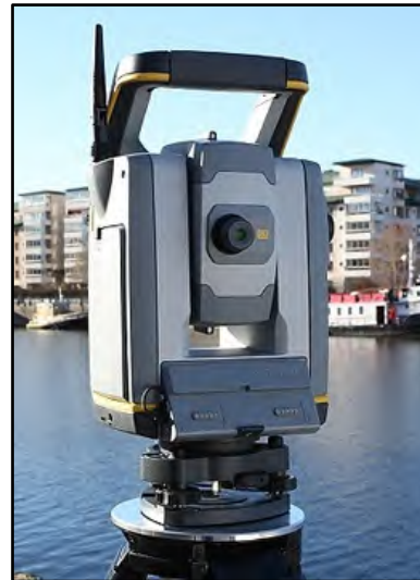
Figure 2.—Backface of Trimble S7 total station should be centered over two tripod legs for efficient leveling.
