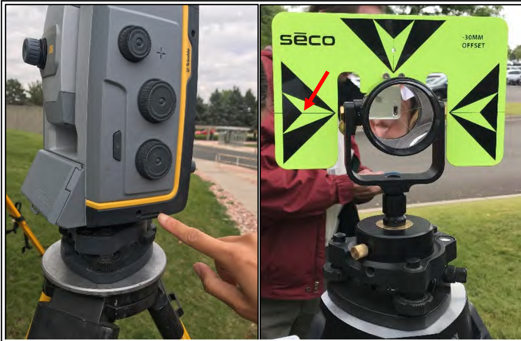
Figures 3 and 4.—Bottom of black notch used to measure antennae height (left) and backsight prism black line used to measure prism height (right).
