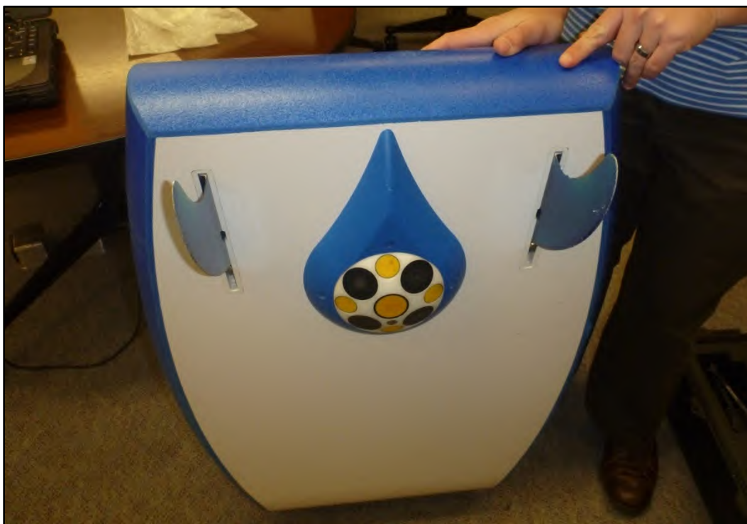
Figure 7.—Install ADCP with 1 to 2 inches of draft between hydroboard and bottom of the ADCP. Note: Do not install blue teardrop as it creates vortices.
