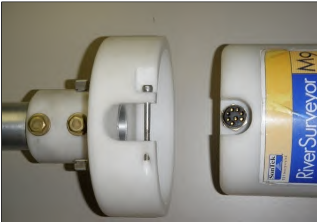
Figure 6.—Remove top mount used for boat if setting up on hydroboard.
